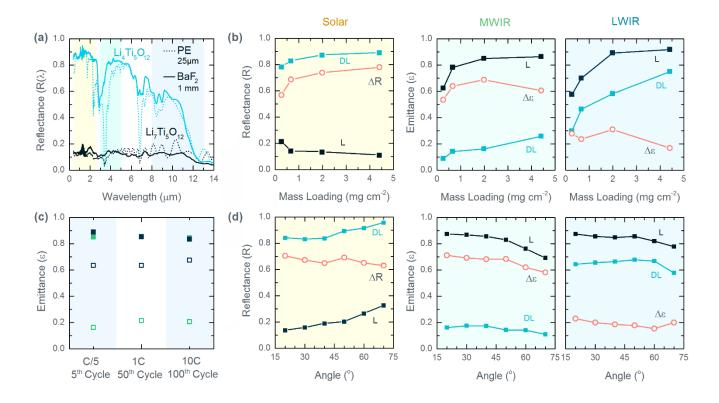
**Figure 2.** Variation of the emittance of the L and DL states of the LTO-based electrodes with (a) type of protective cover (polyethylene (PE) and Barium fluoride (BaF<sub>2</sub>)), (b) mass loading, (c) electrochemical cycling and (d) angle. The background colors in b) and d) represent the solar, MWIR and LWIR atmospheric windows highlighted in
